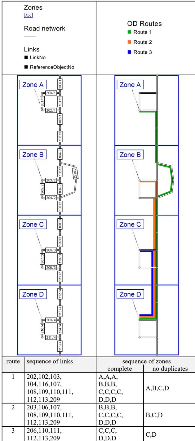
Fig. 4. Identifying potential routes for a matching on the level of traffic zones.
