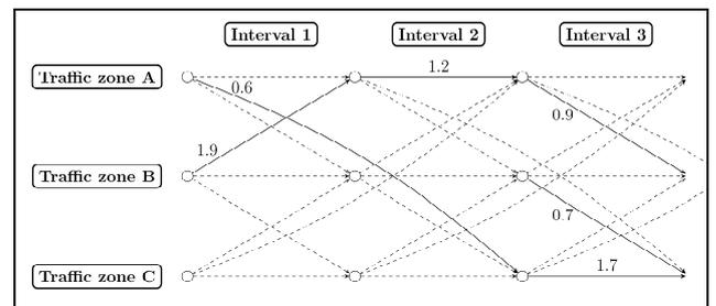
Fig. 5. Example network with three zones and three time intervals. Demanded trips are indicated by solid arcs, the numbers state the amount of vehicles needed.
