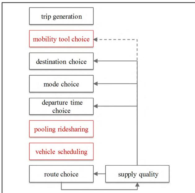
Fig. 2. Extended four-stage algorithm.
