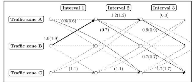
Fig. 6. Vehicle tours for example network of Fig. 5. Solid arcs indicate vehicle tours. Numbers state the demand, numbers in brackets the vehicle flow.
