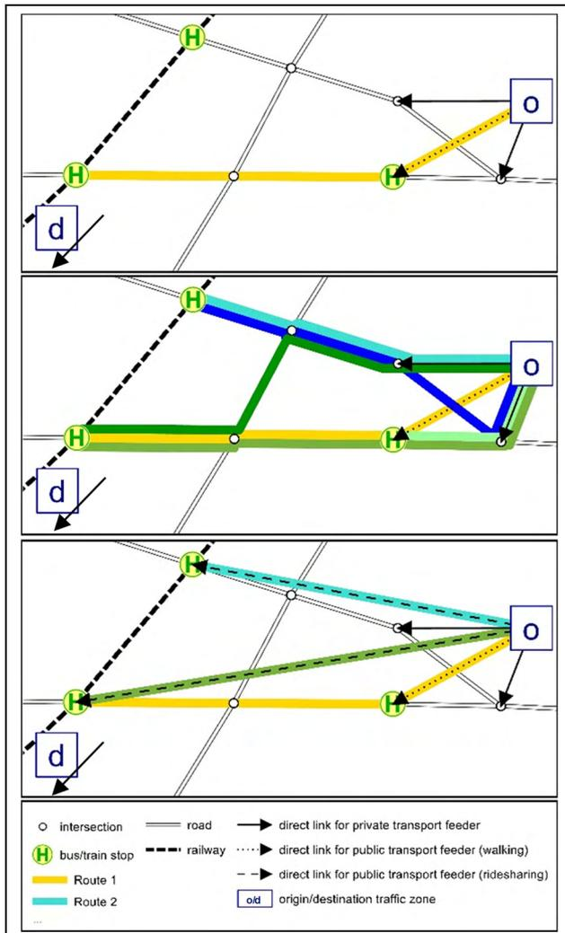
Fig. 3. Example network showing route alternatives for traditional public transport assignment (top), modeling approach A (middle) and modeling approach B (bottom).
