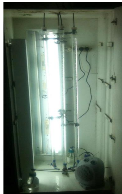
Figure 22. The photo-bioreactors within the temperature controlled cabinet
